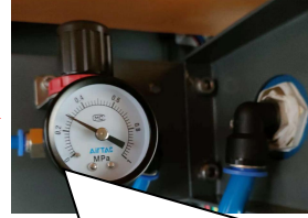
Air pressure requirements 0.3~0.4MPa
